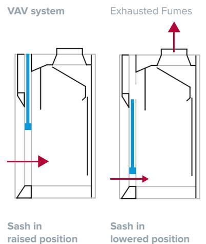
Fan speed continually adjusts to suit sash height, so the required 0.5m/s face velocity is maintained.
