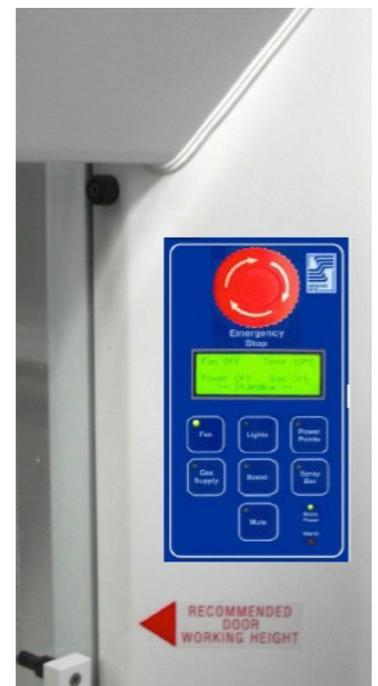
The EcoAir® III Controller comes with a vertically oriented, touch-type control panel that can be mounted on either the left or right column of a fume cupboard. This example shows the control panel mounted on an EcoAir® fume cupboard.
