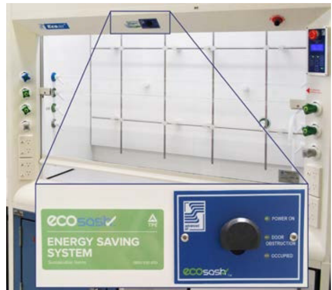
The EcoSash® Motion Sensor module is mounted on the face of the fume cupboard in the centre above the sash. Shown here on an Advanced Air® EcoAir® Fume Cupboard, the sensor panel can be easily mounted on any fume cupboard. It continually monitors activity and communicates with the EcoSash® Controller.
