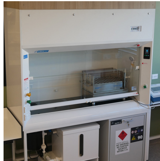
Labrocare® Fume Cupboard with a toxic wet scrubber.
