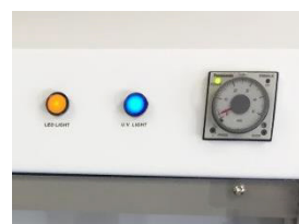
Shown left to right are the LED lighting switch, the UV toggle switch, and the UV Timer.
